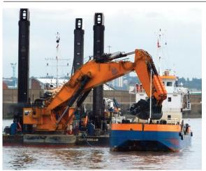
To date we have dredged and disposed of 620m3 of material including stiff clay and silts, some of which was removed using water injection dredging techniques and also by Goliath, one of the largest
